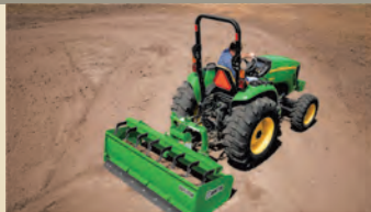
How To Maintain A Gravel Drive Using A Box Blade With Scarifiers
